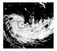
Fig.2 Use of tightest inner curvature compared with linear continuation of band axis.
