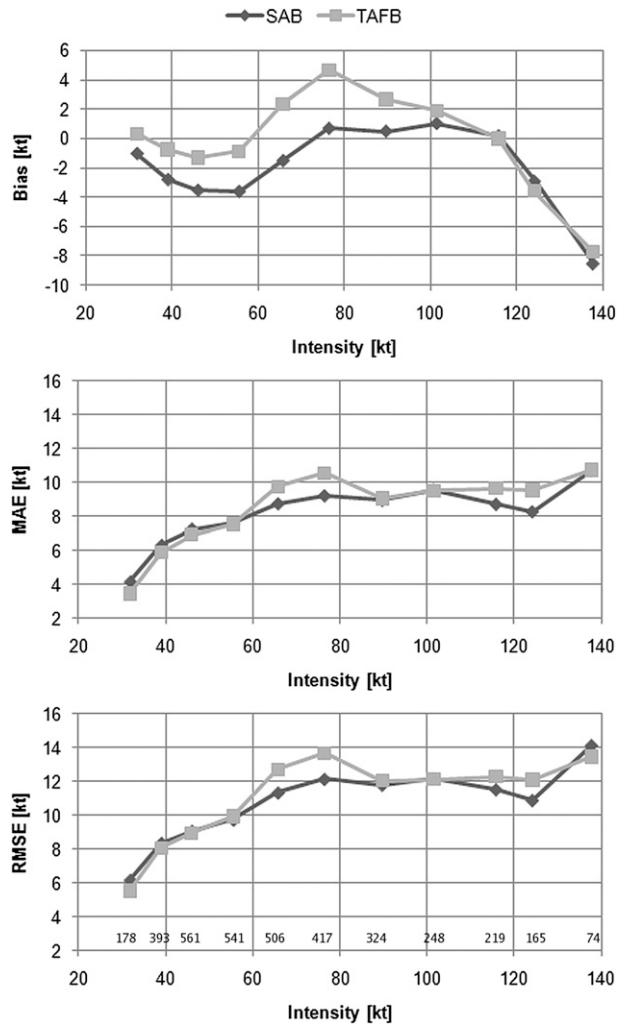
FIG. 3. (top) Biases, (middle) MAEs, and (bottom) RMSEs associated with Dvorak tropical cyclone intensity estimates (kt) from SAB and TAFB that were made with  $\pm 2$  h of an aircraft reconnaissance fix. The verification is based on the best-track intensities at those times, and the analysis domain was the Atlantic basin. The number of cases is provided in the bottom panel.
