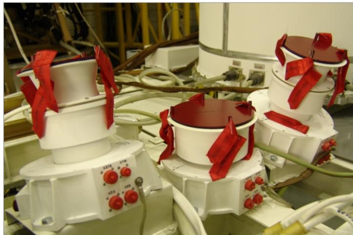
KMSS consists of three cameras. Two of them have a 100mm focal distance, the third one has a 50mm focal distance. Characteristics of both camera types are given below:
